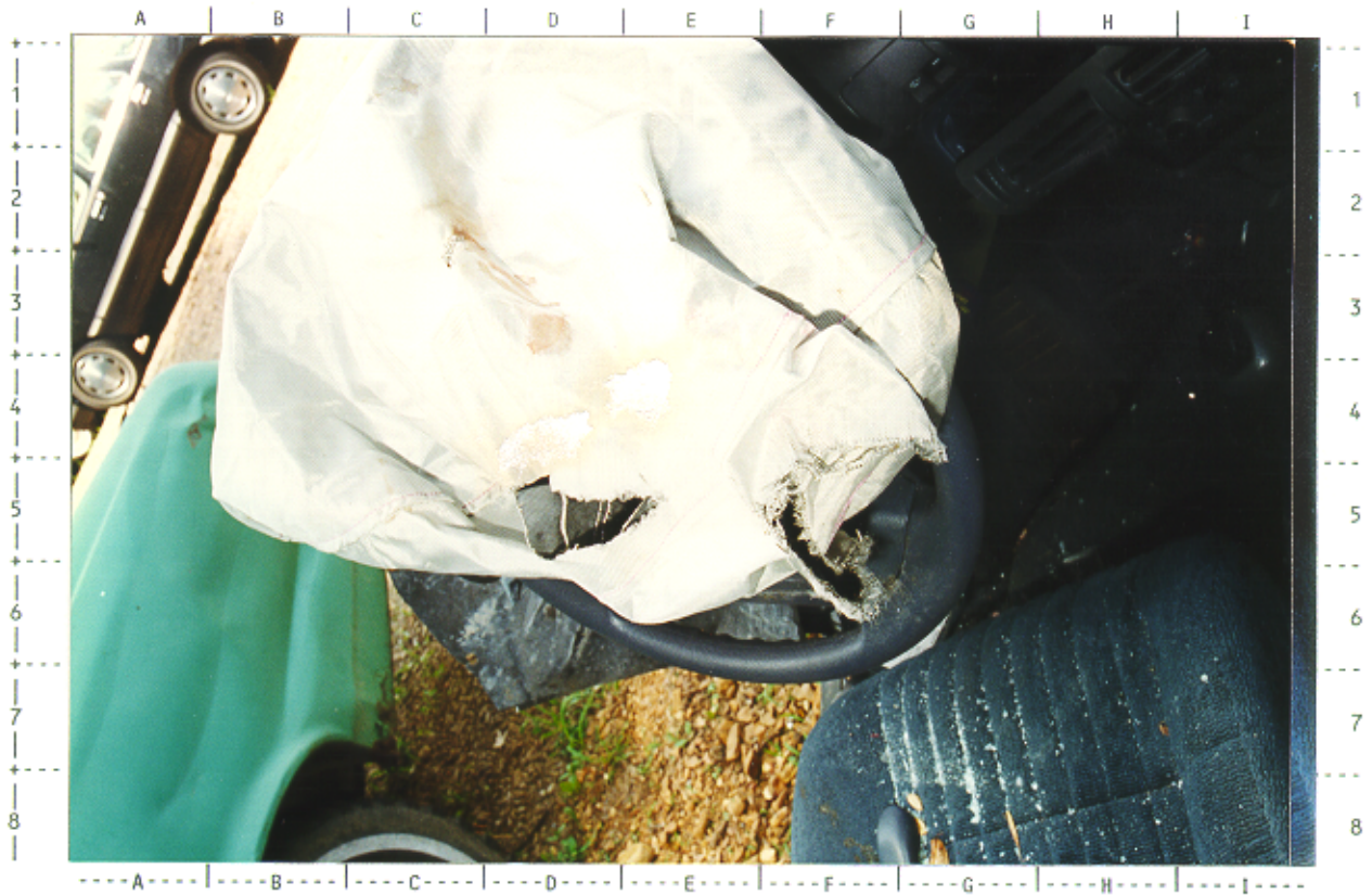
# 55 -- Close-up of underside tears in '91 Corsica's driver air bag most likely from L doors being placed in front seat during towing
